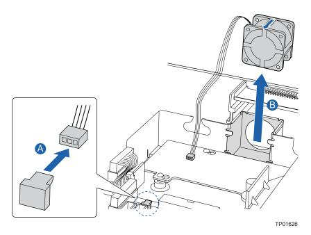
Figure 40. Removing the Single System PCI Fan
